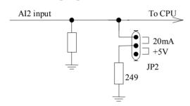
JP2 is used to define the characteristic of the input terminal AI2.
