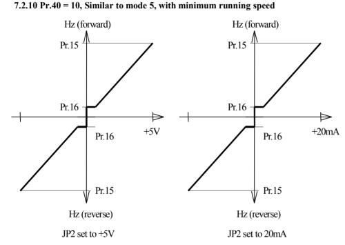
In this mode, the voltage signal fed into AI1 terminal will be used to determine the output frequency and direction of the inverter.
