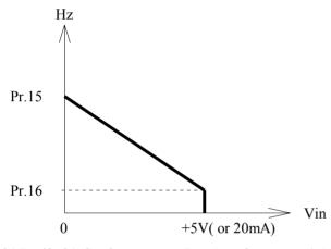
In this mode, the voltage signal fed into AI2 terminal will be used to determine the output frequency of the inverter while running.
