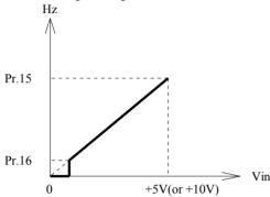
In this mode, the voltage signal fed into AI1 terminal will be used to determine the output frequency of the inverter while running. The direction of the output phase sequence must be determined by control command.
