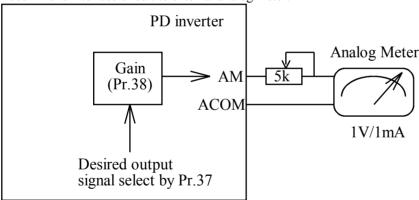
First use Pr.37 to select desired output signal.
