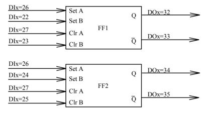
Functional Block diagram of Internal Flip/Flop Modules
