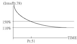
This parameter defines the OVER LOAD trip time of the INTERNAL THERMAL RELAY.
