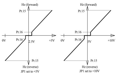
In this mode, the voltage signal fed into AI1 terminal will be used to determine the output frequency and direction of the inverter.
