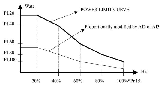
The POWER LIMIT CURVE can be modified by AI2 or AI3, refer to section 8.75.
