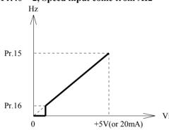
In this mode, the voltage signal fed into AI2 terminal will be used to determine the output frequency of the inverter while running. The direction of the output phase sequence must be determined by
