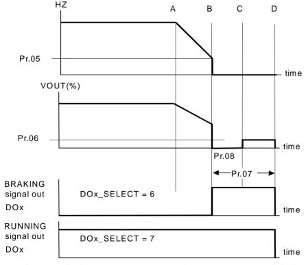
TIMING RELATIONSHIP BETWEEN HZ & VOUT WHILE BRAKING STOP Note:
