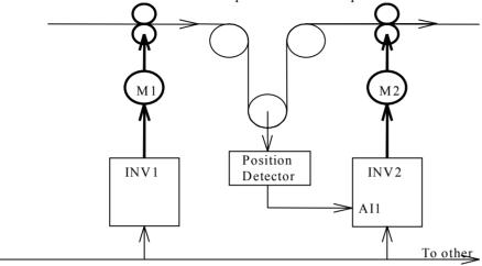
Master Speed Set by KEY-PAD Panel or Computer(from serial port)
