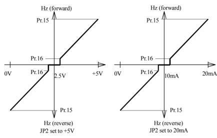
In this mode, the voltage signal fed into AI2 terminal will be used to determine the output frequency and direction of the inverter.
