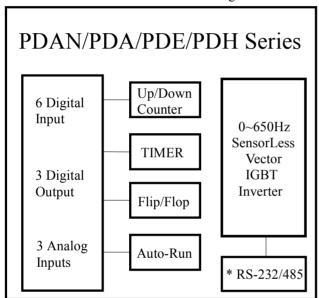
Built in standard **UP/DOWN Counter** Module, **Timer/Counter** Module and **Flip/Flop** Module that are very often used in actual application system.
