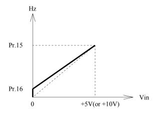
While the desired output frequency is lower than Pr.16 (LOWER LIMIT), the actual output frequency will maintain at the lower frequency limit.
