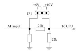
JP1 is used to define the characteristic of the input terminals AI1.
