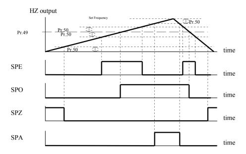
The output status of DOx(2) will **ON**, if the output frequency is **EQUAL** to the preset frequency defined in Pr.49. **Definition of EQUAL** means: Difference is within the allowable tolerance defined in Pr.50.
