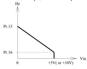
This mode is similar to mode 20, but AII is used instead of AI2. In this mode, the voltage signal fed into AI1 terminal will be used to determine the output frequency of the inverter while running.
