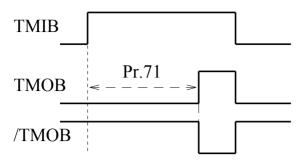
When digital input DIx is assigned to **TMIB** function, it serves as **Input of the ON-DELAY** timer. User must assign a digital output DOx, which select **TMOB** function to serve as the output of this timer. And the **timer time** will be defined in Pr.71. (Refer to Sec.8.94)
