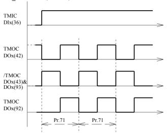
If the input TMIC is OFF, the output TMOC is always under ON state.
