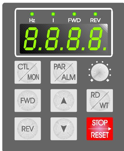
Push the "CTL/MON" key, will change the keypad operation between "CTL" and "MON" Mode. If both "HZ" and "I" Led are blank, it is under "CTL" Mode. Under "CTL" Mode, user can control the driver running in either direction And may modify the desired running speed.
